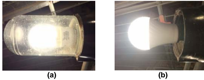
Figure 3. (a) All FL light bulbs were enclosed in glass jars, and (b) some of the LED light bulbs were used without glass jars.
